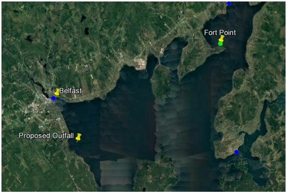
Figure 2. Location of NOAA NOS stations at Belfast (8415191) and Fort Point (8414721), and approximate location of proposed outfall.
